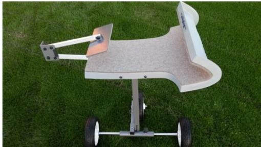
Wing Rigger was the first commercial rigging system offering a gas spring assist. The gas spring, located inside the main column, pushes upward on the wing saddle with a continuous lifting force related to the pressure in the gas spring.
