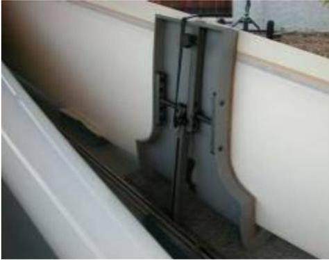
Some pilots store the saddle assembly in the aft part of their trailer for convenient access. One strategy is to place the saddle in its upright position around the wing itself as pictured here. This often works well for gliders with swept back leading edge (an ASW-27 is shown). You'll want to use sufficient elastic bands or other attachment to make sure that the saddle can't shift position on a bumpy road.
