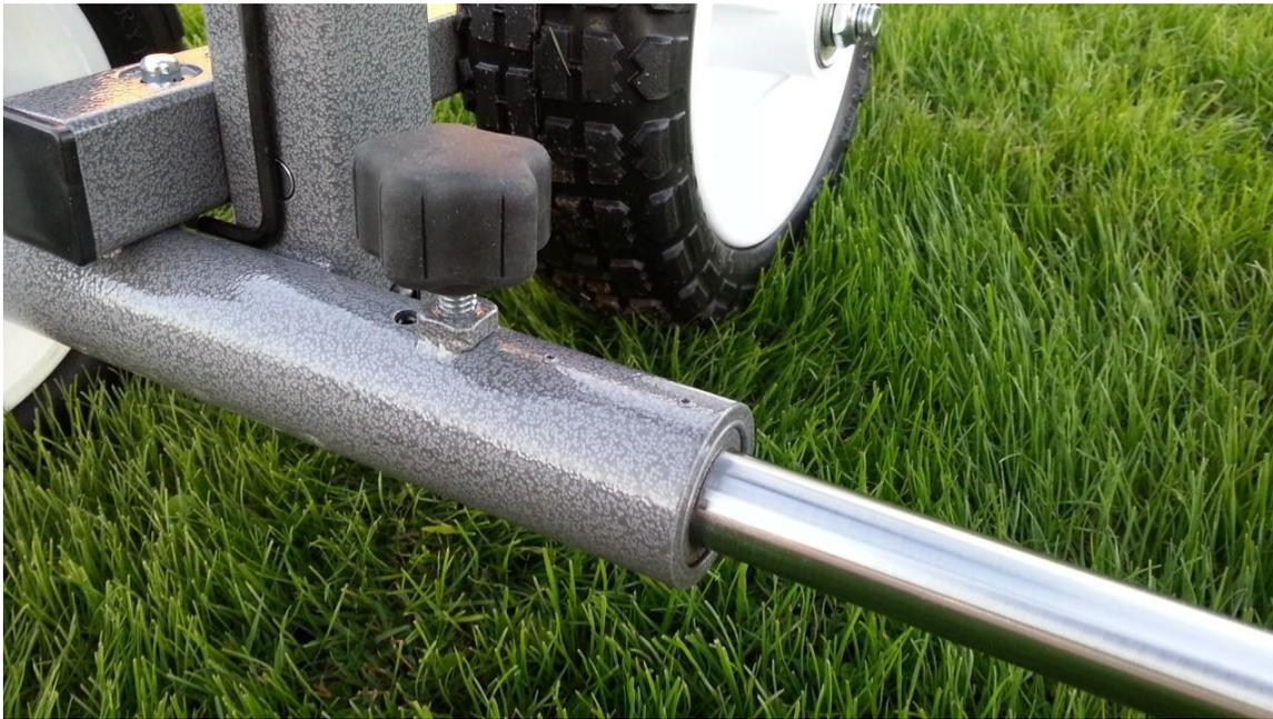
Wing Rigger operates on three wheels. The two outer wheels carry the running load while the center wheel is offset vertically and functions primarily like a rolling ‘kick stand’. When the unit is loaded with a glider wing, this center wheel is automatically lifted off the ground as the Wing Rigger is leveled by its payload.
